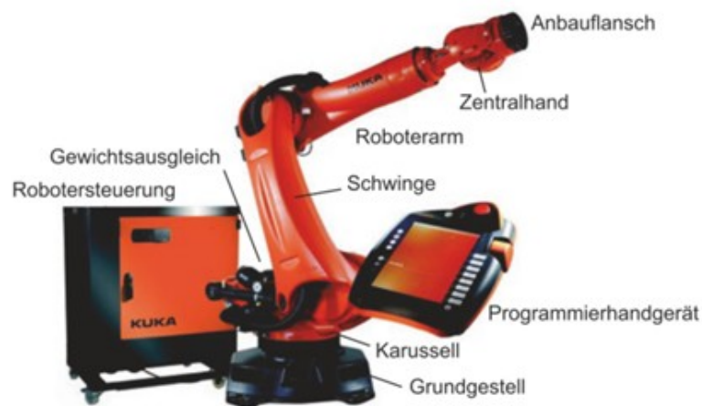
Figure 14.1: Construction of a six-armed articulated robot
