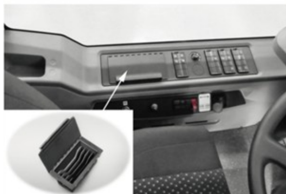
Figure 15.13: Money tray: Additively manufactured by Daimler
