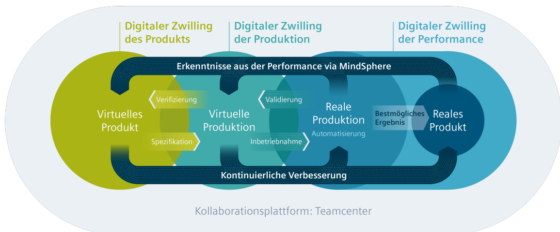
Figure 7.3: Types of digital twin and their connection to the real product [20].
