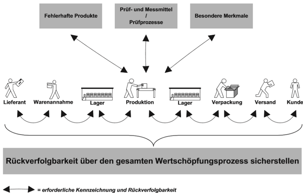
Figure 10.6: Marking and traceability along the value creation process
