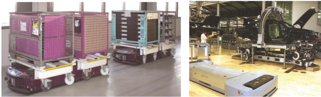
Figure 10.9: Left: underride AGV with small roller carts for mesh boxes; right: assembly AGV at Volkswagen; in the background, the drivetrain and body are being married on an AGV, while an empty AGV moves away in the foreground
