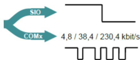
Figure 11.3: Operating modes of IO-Link
