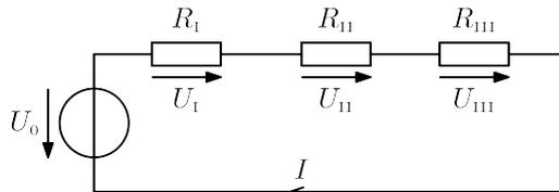
$$R_{ges} = R_I + R_{II} + R_{III} \quad \text{mit:} \quad R_I = R$$
